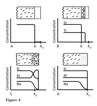
Illustration of different corrosion processes on a glass surface (51). (A) Congruent dissolution releases all elements at a single rate, (B) incongruent dissolution releasing elements at different rates, (C) corrosion of surface by chemical reaction of solvent with solid, and (D) leaching of alkali without affecting network elements.
